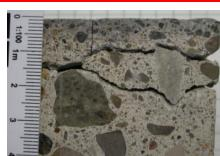
These delaminations become apparent within the first few weeks after slab placement, are approximately 10-20 mm in depth and vary from 600 mm in size to full bays. These problems seem to relate to a combination of:
